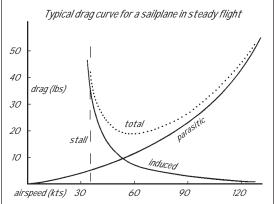
the trailing vorticity is spread out more as well, dissipating less energy. If the aircraft flies faster, it produces the same lift with less angle of attack, less disturbance to the flow, and creates weaker vorticity in the trailing wake.
